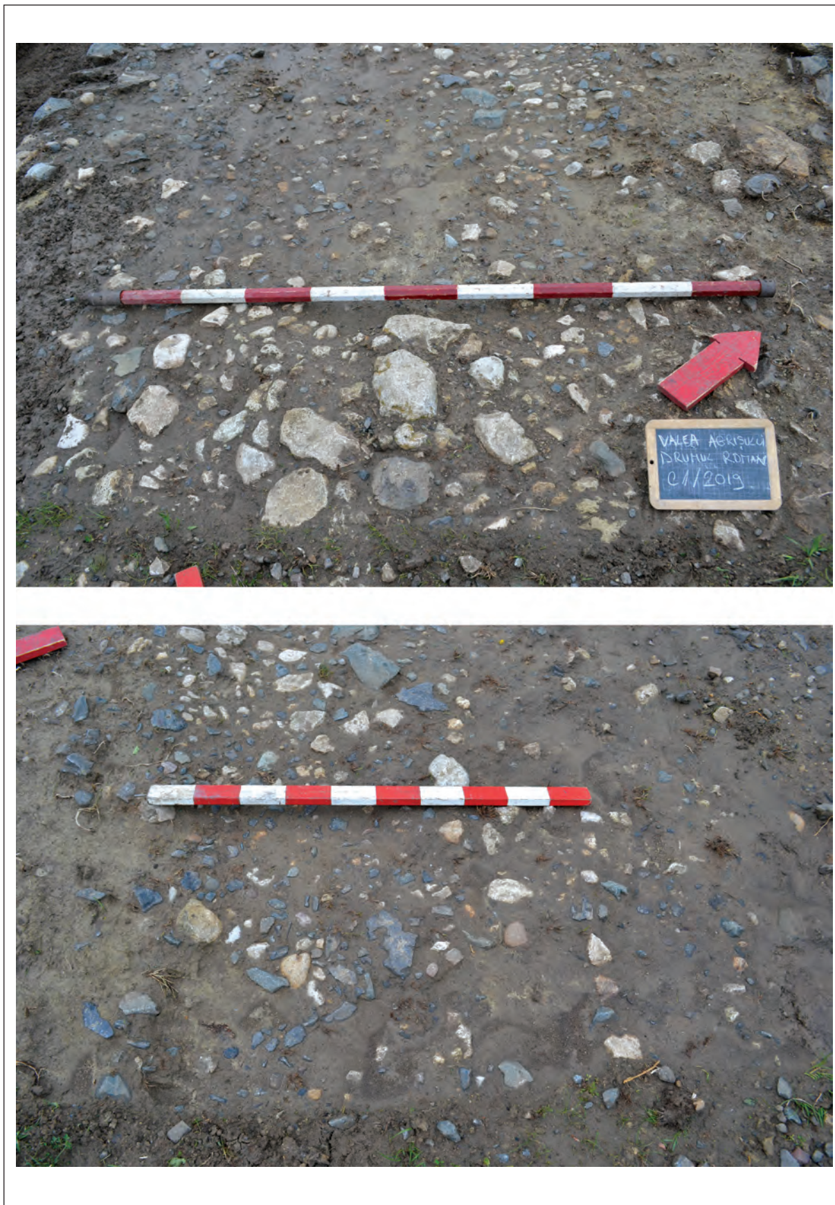
Pl. 5. Ftr. 2-the pavimentum and Ftr. 3-the rudus of the road.
